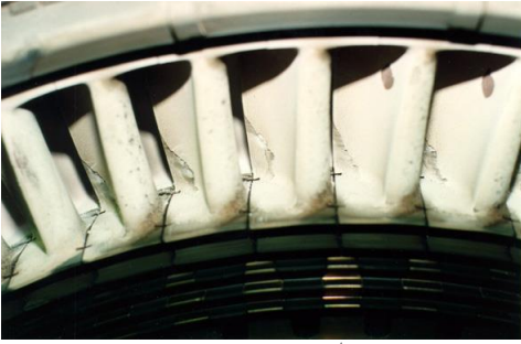
Figure 12. High Pressure Turbine 1 st rotor blades (Stamatis et al., 1999)
