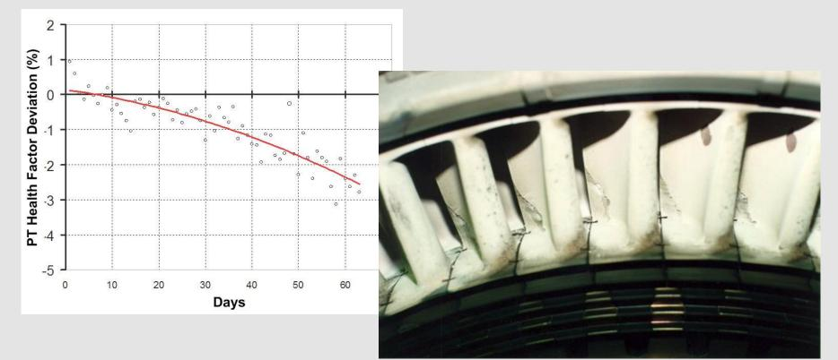
Fault : Deposits on both gas generator and power turbine blades due to anticorrosive additives of the fuel
