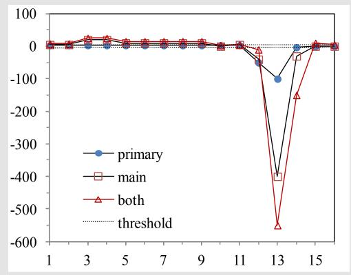
Temperature patterns are obtained from sensors placed at certain circumferential locations that correspond to a discrete spatial sampling of the continuous temperature distribution.
