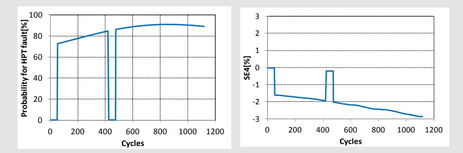
The method of PNN estimates that an increasing HPT fault occurs The deterioration tracking method detects an increasing deviation of HPT efficiency
