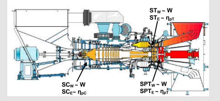
Application of the adaptive performance modeling technique on an Industrial GT in cooperation with the Operator for Fault Identification by post processing of Engine Measurements
