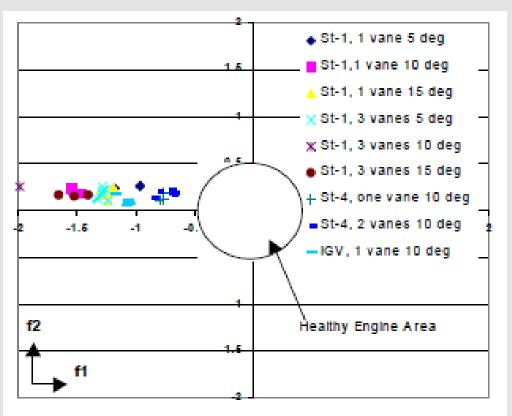
A decrease in compressor pumping capacity is detected, while its efficiency remains practically unaltered.
