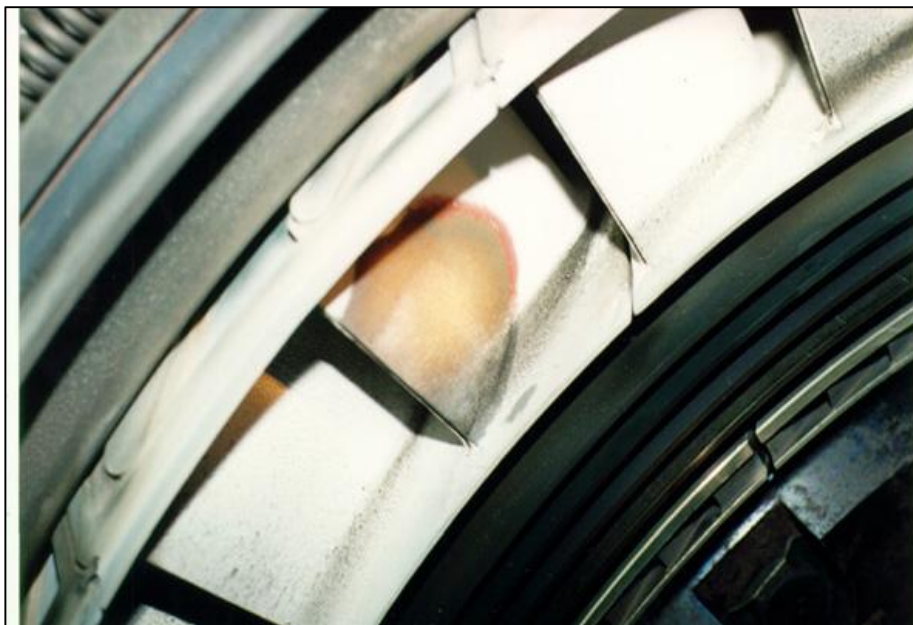
Compressor Turbine 1 st Stator vanes. Suction side view.
