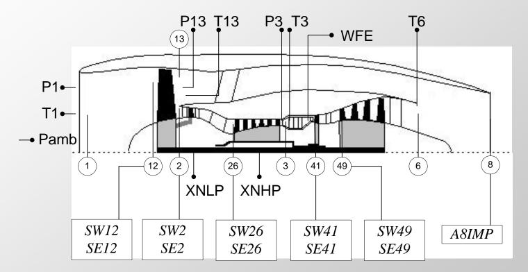
High-by-Pass ratio, partially mixed, turbofan engine used as a test case
