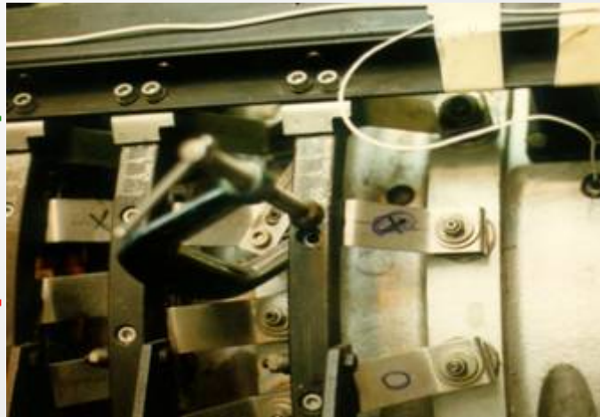
Mistuned stator vanes
