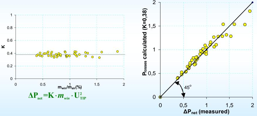
•The losses can be attributed to the centrifugation of the droplets by the Rotor
