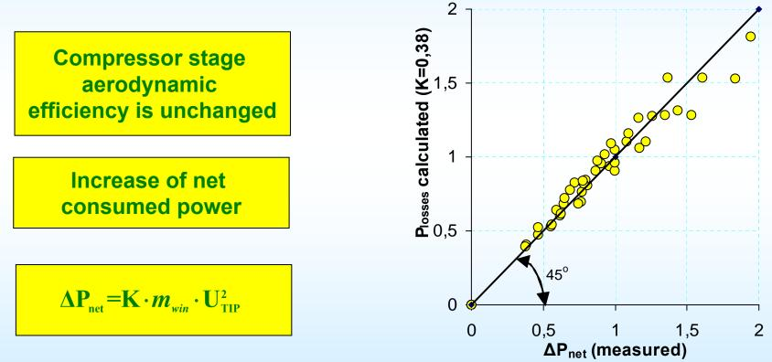
•The losses can be attributed to the centrifugation of the droplets by the Rotor
